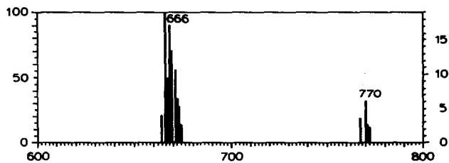
Fig. 3. FD-mass spectrum of \text{PdMo}(\mu\text{-Ph}_2\text{Ppy})_2(\mu\text{-CO})(\text{CO})_2\text{Cl}_2 .
